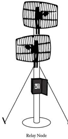
Figure 8. Sketch of an access- and relay node.
